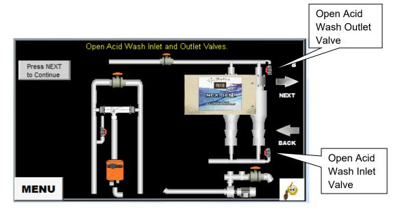
STEP 9 – Open both White Acid Wash Valves on the Acid Wash assembly.
