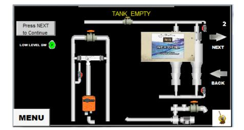
**STEP 3** – Open Tank Fill Valve marked 3.
