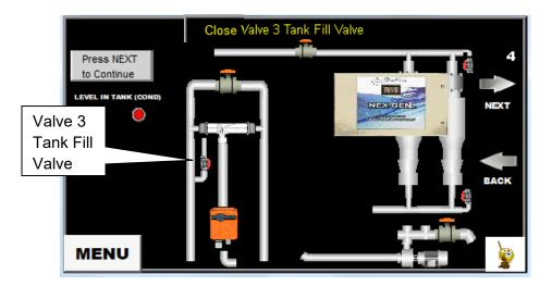
**STEP 5** – The system will flush and drain the tank. When flushing and draining is complete, the Low Level Sw will turn from GREEN to RED and the display will prompt you to Press NEXT to continue.
