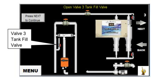
**STEP 4** – This step will fill the tank for flushing. When the tank is full the RED Level In Tank (Cond) will turn GREEN and the display automatically changes to the screen on the next page.
