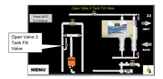
**STEP 23** – This step will fill and flush the system. Once filling and flushing is complete, the current system pH will be displayed and you will be prompted to press NEXT to continue.
