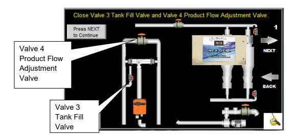
**STEP 2** – During this step the booster pump will start and the product tank will empty. When the tank is empty the GREEN Low Level Sw will turn RED.
