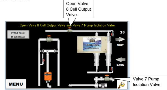
**STEP 21** – This step will empty any remaining acid from the cells. When the process is complete the Press NEXT to continue prompt will allow you to move to the next step.
