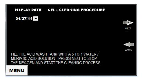
**Note:** Sulfuric acid and dry acid (sodium bisulfate) are not recommended for cell cleaning. Under some conditions the electrolytic cell can be damaged.
