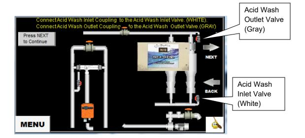
**STEP 8** – Open the Acid Wash Inlet and Outlet Valves.
