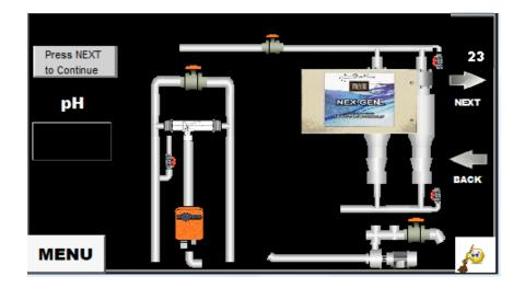
**STEP 24** – Adjust the Production Flow Valve marked 4 to the desired flow rate outlined in Section 3.2 on page 16.
