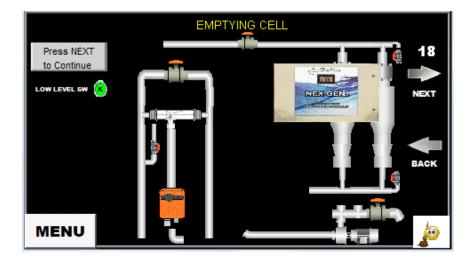
**STEP 19** – Open Valve 3 the Tank Fill Valve.
