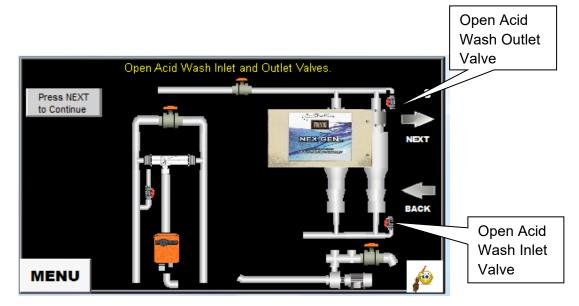
STEP 6 – Open both White Acid Wash Valves on the Acid Wash assembly.
