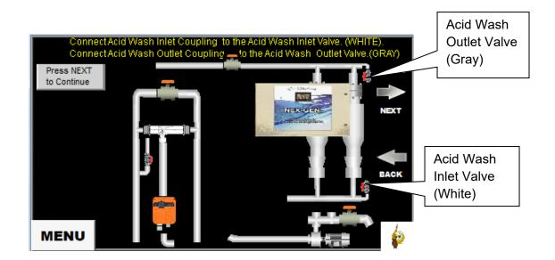
**STEP 5** – Open the Acid Wash Inlet and Outlet Valves.
