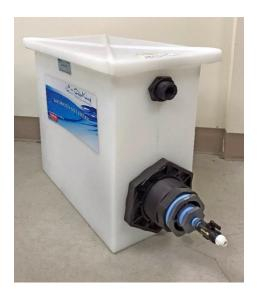
Plumb the peristaltic pump suction line to the salt outlet on the Saturated Salt Feeder with 1/4 tubing supplied with the peristaltic pump. The salt outlet on the Saturated Salt Feeder is a small blue and white valve located at the bottom of the salt feeder. Plumb the Saturated Salt Feeder water supply to the fitting on the chemical metering assembly using  $\frac{1}{2}$  inch tubing.
