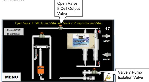
**STEP 18** – This step will empty any remaining acid from the cells. When the process is complete CELL EMPTY will be displayed.
