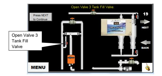
**STEP 20** – This step will fill and flush the system. Once filling and flushing is complete, the current system pH will be displayed and you will be prompted to press NEXT to continue.
