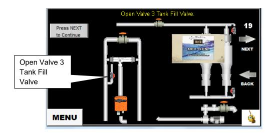
**STEP 20** – This step will fill and flush the system. Once filling and flushing is complete, the current system pH will be displayed and you will be prompted to press NEXT to continue.
