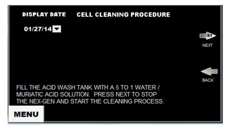
**Note:** Sulfuric acid and dry acid (sodium bisulfate) are not recommended for pH adjustment. Under some conditions the electrolytic cell can be damaged.
