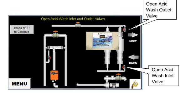
STEP 6 – Open both White Acid Wash Valves on the Acid Wash assembly.
