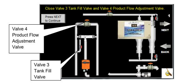
**STEP 2** – During this step the booster pump will start and the product tank will empty. When the tank is empty the GREEN Low Level Sw will turn RED.
