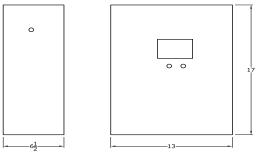
Keep 32" clear above this point to allow for 5 removal of quartz sleeve 3<u>5</u> 16  $49\frac{15}{16}$  $28\frac{7}{16}$  $42\frac{5}{16}$  $7\frac{15}{16}$ -11 -14<mark>5</mark>
